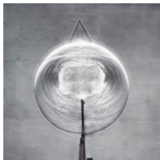
Figure 1. Muzzle Blast from a Rifle (Settles, 2006) High Speed Imaging of Shockwaves
